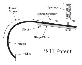
hinge plate upwards to urge the shoe into the ground but compressed to allow pivoting movement of the hinge plate about the pivot axis in response to the shoe hitting a rock.<sup>113</sup>
