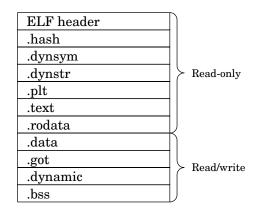
An ELF dynamically linked program looks much like an ELF shared library. The main difference is that a dynamically linked program has an INTERP section near the beginning of the file so the name of the dynamic linker to be used to load the file can be specified.<sup>115</sup> Additionally, a dynamically linked program does not have a ".got" section, because program files are not relocated at run-time.<sup>116</sup>
